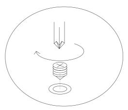
rotate Cam grub screw into the cam sleeve and tighten
