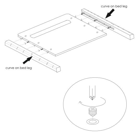
rotate Cam grub screw into the cam sleeve and tighten
