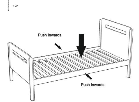
Some "light" inward pressure on both rails before screwing down the bed laths helps keep the bed parallel
